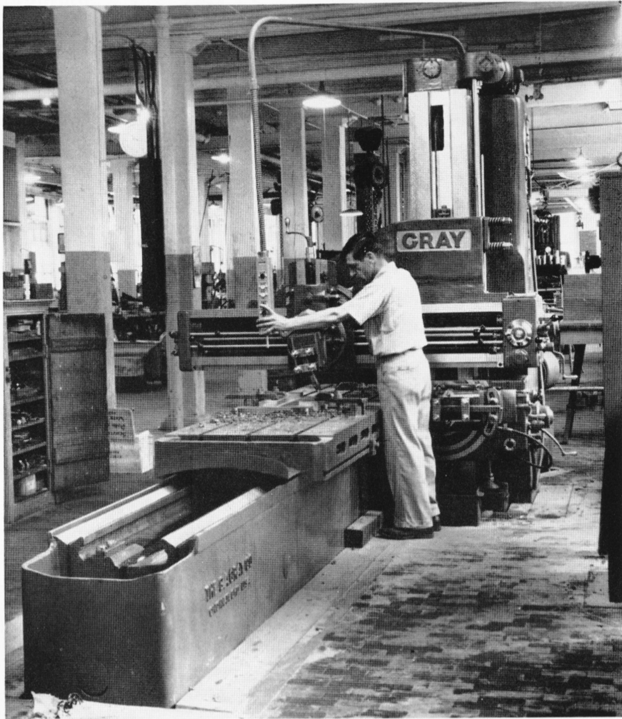
Valmore Bernier operates the new Gray Planer which has been installed in the West Machine Room recently. This machine has been designed for heavy cutting with high speed carbide tools and will provide production, convenience and rigidity with Tool Room precision and versatility.
